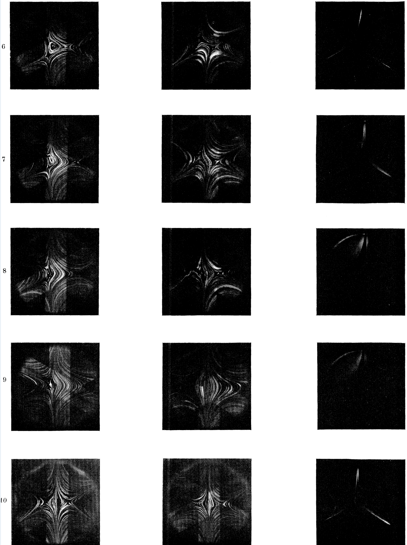
FIGURE 8. Streamline patterns of (a) glycerol and (b) 2% polyethylene oxide solution in the six roll mill corresponding to roller speeds \Omega_I , \Omega_{II} and \Omega_{III} of table 2. (c) Corresponding flow birefringence observations of the polyethylene oxide solution.
